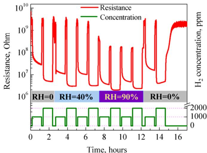
Fig. 4. Long-term testing of hydrogen sensor operation in different RH levels conditions.
