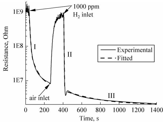
Fig. 3. Transients of sensor response to 1000 ppm H<sub>2</sub> and recovery in air (at 150°C operating temperature).
