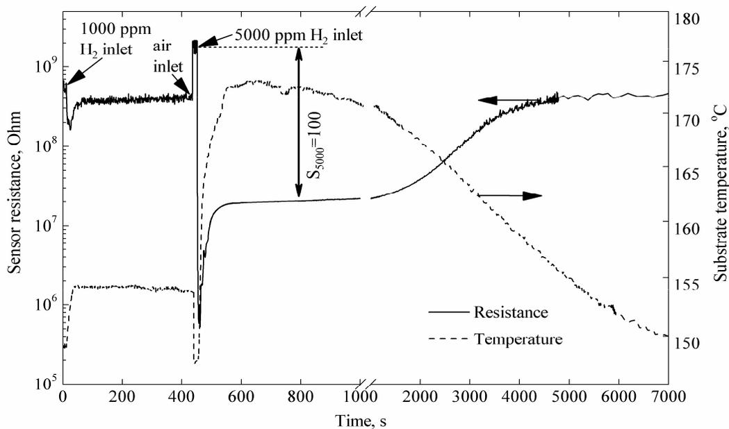
Fig. 1. Plots of hydrogen sensor resistance and substrate temperature with time in initial stage of the long-term treatment.
