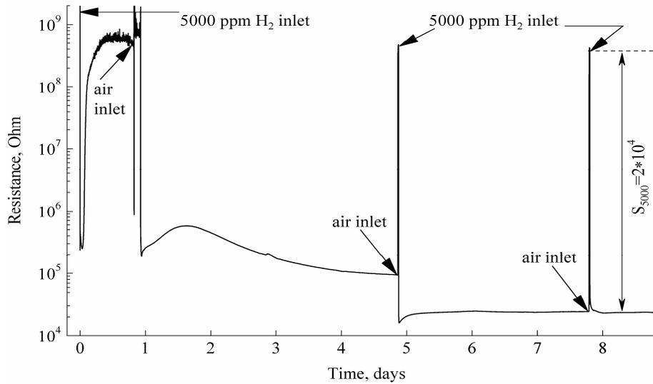
Fig. 2. Hydrogen sensor resistance changes during long-term exposure in hydrogen containing environment at operation conditions.
