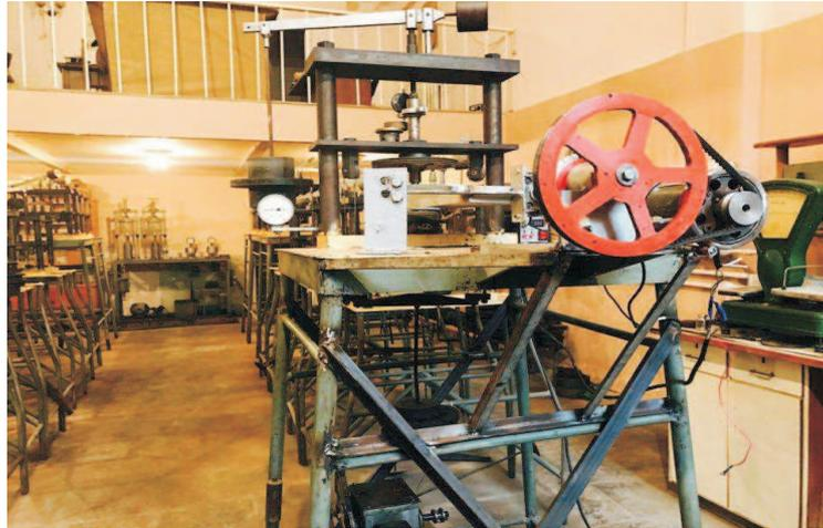
**Figure 2.** Upgraded M-5 torsion test tool.
