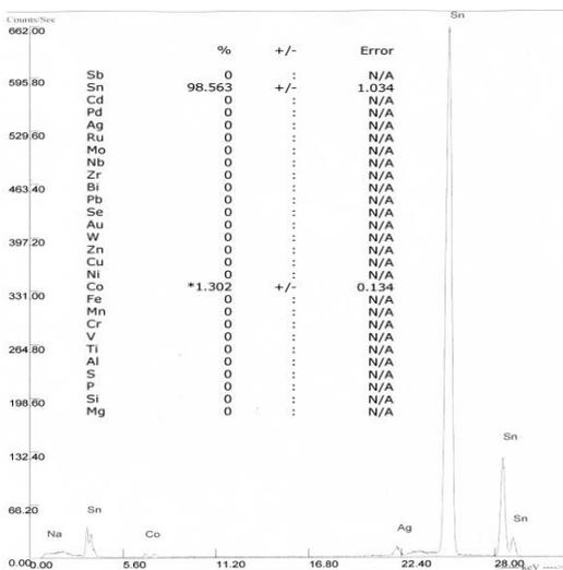
Fig. 1. The result of chemical analysis of the  $\text{SnO}_2\langle\text{Co}\rangle$  target.
