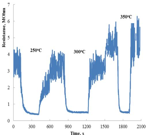
Fig. 4. The SnO<sub>2</sub><Co> sensor resistance variation under the influence 200 ppm of dichloromethane at different work body temperatures.
