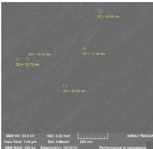
Fig. 3. The SEM image for the  $\text{SnO}_2\langle\text{Co}\rangle$  films.
