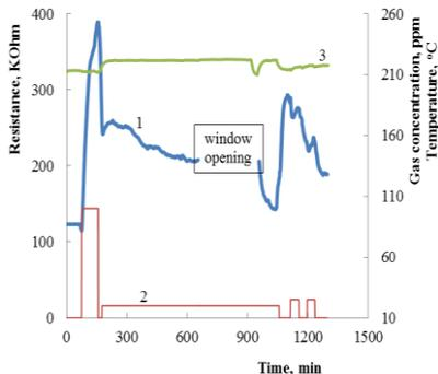
Fig. 7. The resistance variation under influence of yperite for Co-doped SnO<sub>2</sub> sensor (1). Curves (2) and (3) - gas concentration and work body temperature, accordingly.
