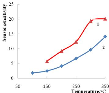
Fig. 5. The SnO<sub>2</sub><Co> sensor sensitivity dependence on temperature to 500 ppm dimethylformamide (1) and 350 ppm dichloroethane (2).
