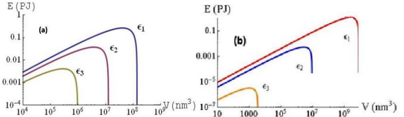
Fig. 2. Dependence of the GaInAlN composition islands energy on volume at different strain for zinc-blend and wurtzite symmetry at different strain ( $\epsilon_1 = 0.02$ ,  $\epsilon_2 = 0.025$ ,  $\epsilon_3 = 0.03$  and  $\epsilon_1 = 0.004$ ,  $\epsilon_2 = 0.008$ ,  $\epsilon_3 = 0.01$ ), respectively.
