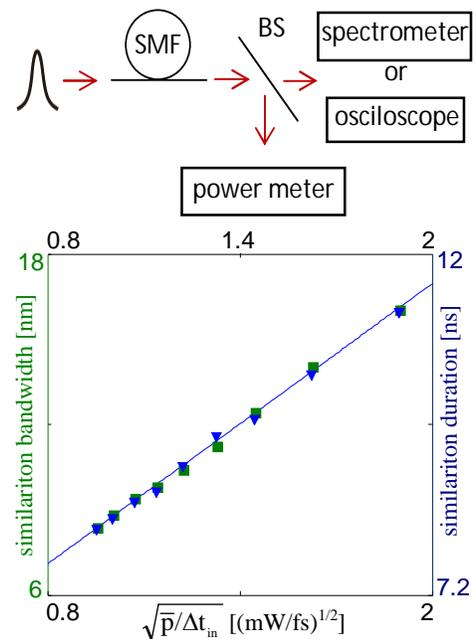
Fig. 1. Experimental results of duration measurements for chirped laser pulses. The similariton bandwidth (green squares, left axis) and similariton duration (blue triangles, right axis) versus  $\sqrt{\bar{p}/\Delta t_{in}}$ .
