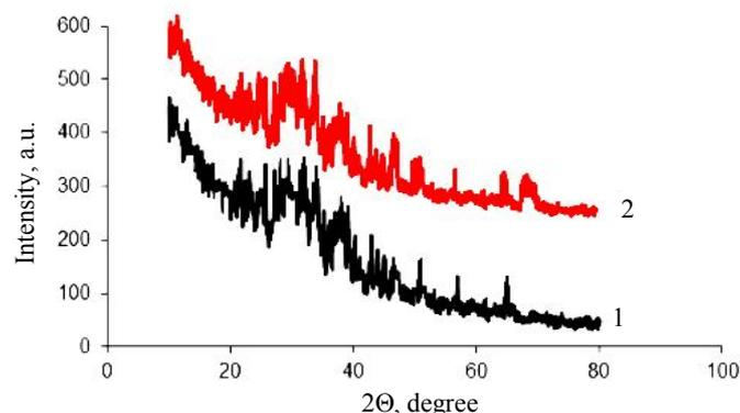
Fig. 1. The diffractograms of samples: 1 – STTP; 2 – STTP peroxy solvate.
