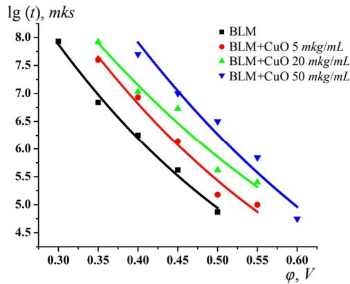
Decrease in the mean lifetime of BLM with increasing voltage in the presence of nanoparticles CuO with concentrations of:
