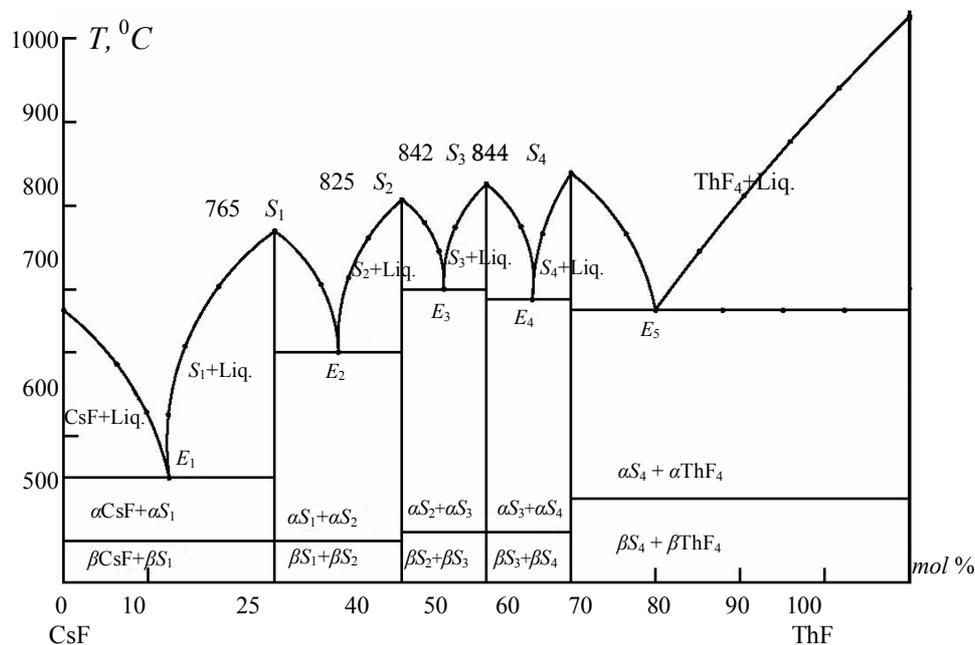
Fig. 1. Diagram of the system's meltability  $\text{ThF}_4\text{-CsF}$ :
