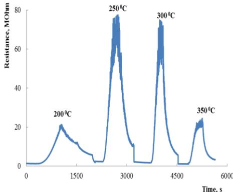
Fig. 3. The resistance variation of the ZnO<La> (80nm) sensor under the influence 1800 ppm of  $H_2O_2$  vapors at different work body temperatures.
