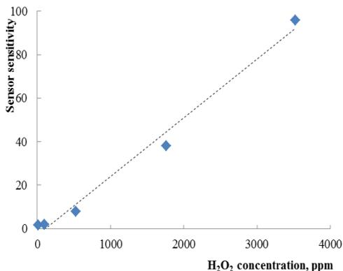
Fig. 7. The sensitivity dependence on H<sub>2</sub>O<sub>2</sub> vapors concentration at operating temperature 220 °C.
