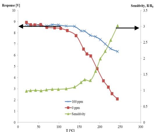
Fig. 5. The temperature dependence of sensitivity to 100 ppm  $H_2O_2$  vapors for ZnO<La> sensor.
