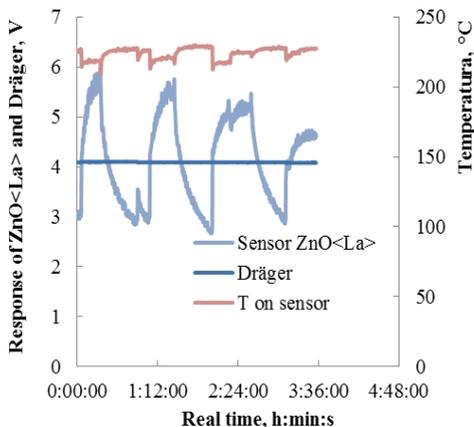
Fig. 6. ZnO<La> sensors response to 10 ppm of H<sub>2</sub>O<sub>2</sub> vapors, work body temperature 220°C.
