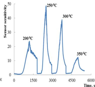
Fig. 4. The ZnO<La> (210 nm) sensor sensitivity to 1800 ppm of  $H_2O_2$  vapors at different work body temperatures.
