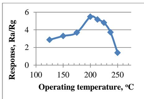
Fig. 1. Response of MWCNTs/SnO<sub>2</sub> thick-film FA sensors vs operating temperature.
