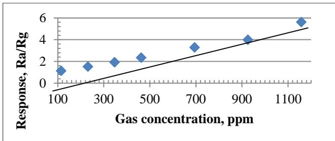
Fig.4. Dependence of the response of MWCNTs/SnO<sub>2</sub> FA vapor sensor on gas concentration measured at 200°C operating temperature.
