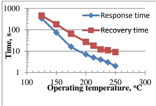
Fig. 2. Dependence of the response and recovery times of MWCNTs/SnO<sub>2</sub> FA vapor sensor on operating temperature.
