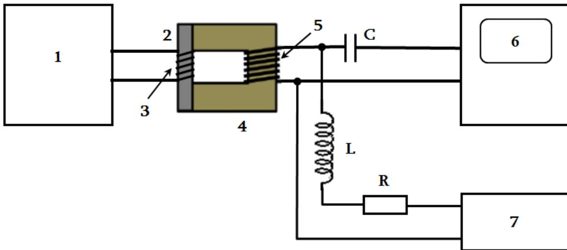
**Figure 1.** The experimental setup: 1. Microwave sweep generator, 2. YIG sample, 3. Primary coil, 4. Horseshoe shaped ferrite, 5. Secondary coil (for sensing and bias magnetization), 6. Oscilloscope, 7. Adjustable DC source, C – decoupling capacitance, L – decoupling inductor, R – ballast resistor.
