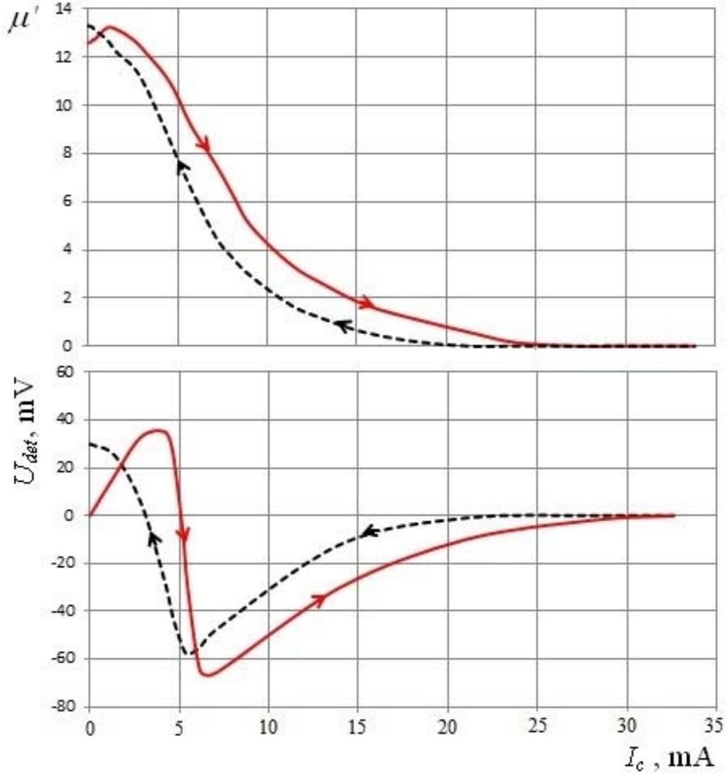
Fig.2. The dependence of differential magnetic permeability and the magnitude of the detected signal on bias current of magnetizing coil 5 (the solid lines – at increasing of the bias current, dash line - at decreasing of the bias current).
