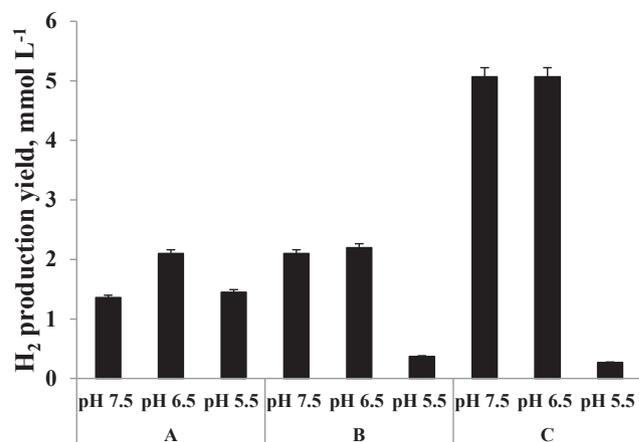
**Fig. 4** –  $H_2$  production by *E. coli* BW25113 in the presence of acetate at different pHs. For others see [Materials and methods](#) and legends to [Fig. 1](#).
