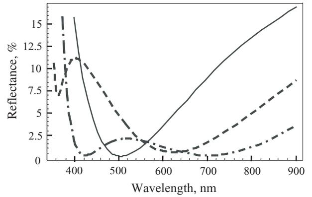
**Figure 3.** Reflectance spectra of single layer DLC (—) and DLC/PS double layer coatings: ( $n_{\text{DLC}} = 1.6$ ;  $n_{\text{PS}} = 2.9$ ;  $d_{\text{DLC}} = 85$  nm;  $d_{\text{PS}} = 30$  nm, ·····) and ( $n_{\text{DLC}} = 1.6$ ;  $n_{\text{PS}} = 2.8$ ;  $d_{\text{DLC}} = 86.9$  nm;  $d_{\text{PS}} = 47.9$  nm, — · —).
