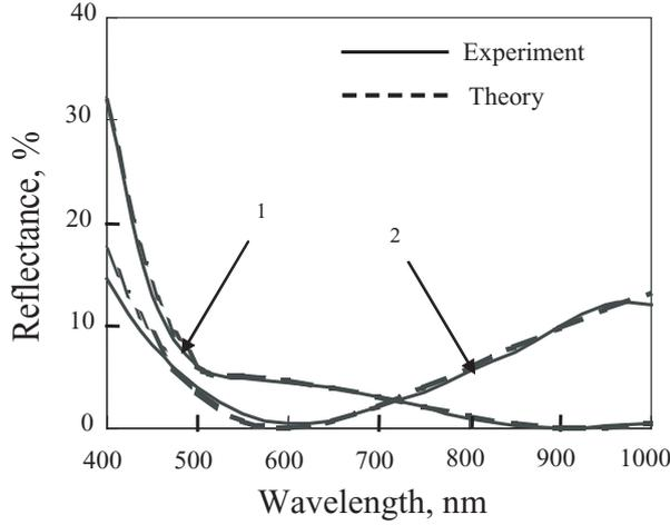
**Figure 1.** Experimental and calculated reflectance versus wavelength of the MgF<sub>2</sub>/ZnS (1) and SiO<sub>2</sub>/TiO<sub>2</sub> (2) double layer coatings.
