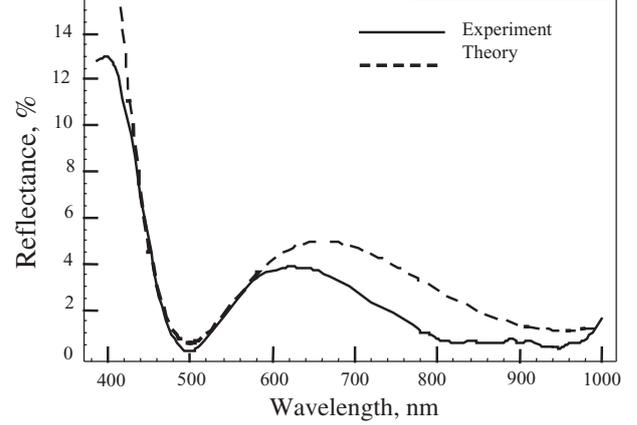
**Figure 2.** Simulation of the reflectance of a PS penta-layer.
