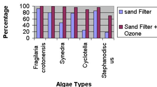
Comparison of Algae control with only filtration system versus a combination of ozonation and filtration systems.
