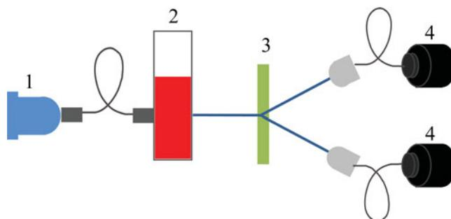
**Figure 5.** Experiment scheme of circular dichroism measurement of vitamin B12: 1 – LED (425 nm); 2- cuvette with sample; 3-Circular diffraction waveplate; 4- light intensity controllers SN P2001297 (ThorLabs).
