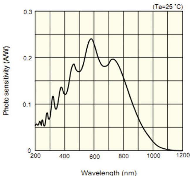
**Figure 2.** Spectral sensitivity of S3903-1024Q linear sensor.
