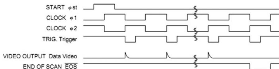
**Figure 4.** Control signals generated by programmable logic device.
