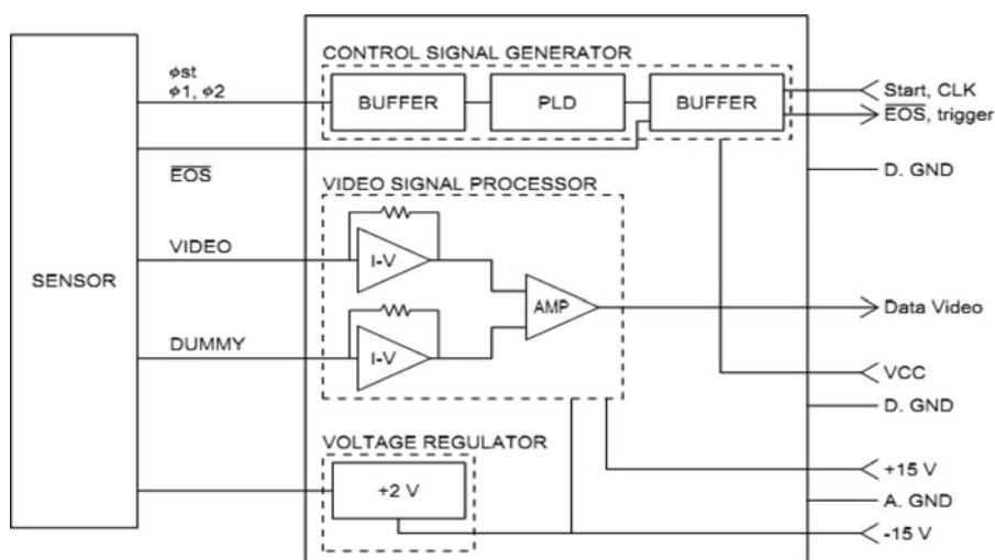
**Figure 3.** Block-diagram of driver circuit.
