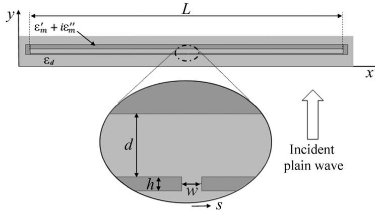
**Fig. 1.** Scheme of the cross-section of structure. The dark area is filled with the silver, while the rest is filled with a dielectric medium with the permittivity  $\epsilon_d$ , where  $s$  is a shift of the slit center from the center of the cavity resonator.
