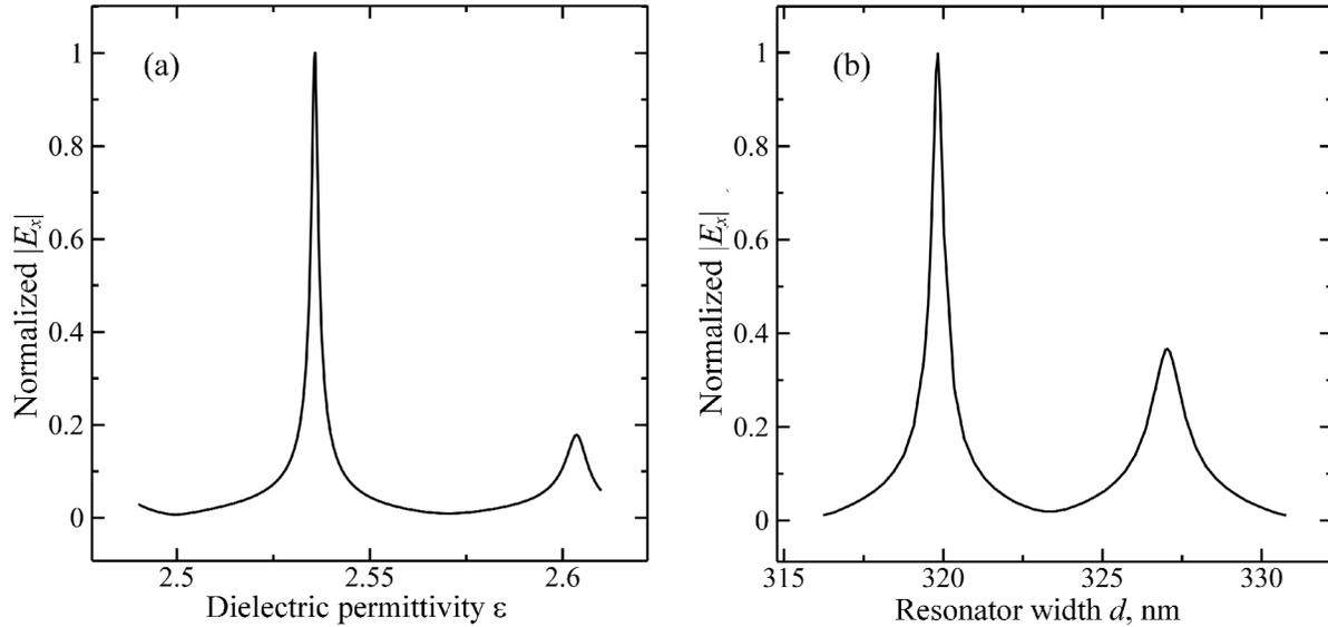
**Fig. 4.** Dependence of the absolute value of the amplitude  $E_x$  in the resonator on (a) the relative dielectric constant of the medium and (b) the width  $d$  of the resonator. The resonator length is  $L = 20000$  nm, the width  $d = 316$  nm, the size of the slit  $w = 100$  nm, the height of the lower metal  $h = 70$  nm, the slit shift from the center of resonator  $s = 0$  nm, and the wavelength 1000 nm.
