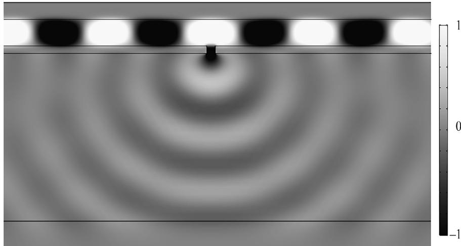
**Fig. 2.** The field component  $E_x$  excited at the resonance wavelength 1008.75 nm by the subwavelength slit in the silver plate of a plane-parallel resonator. The length of resonator is  $L = 20000$  nm, the width  $d = 316$  nm, the slit size  $w = 100$  nm, the thickness of the lower metal layer  $h = 70$  nm, the shift of slit from the center of the resonator  $s = 0$  nm and the permittivity of the medium  $\varepsilon_d = 2.5$ .
