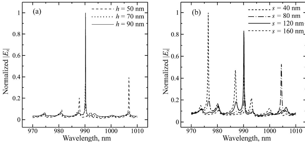
**Fig. 3.** Dependence of the absolute value of the amplitude  $E_x$  in the resonator on the wavelength for (a) the different values of  $h$ , when the shift of the slit from the center of resonator  $s = 120$  nm, and (b) at the different  $s$ , when the height of the lower metal  $h = 70$  nm. The length of the resonator  $L = 20000$  nm, the width  $d = 316$  nm, and the size of the slit  $w = 100$  nm, the permittivity of the medium  $\epsilon_d = 2.5$ .
