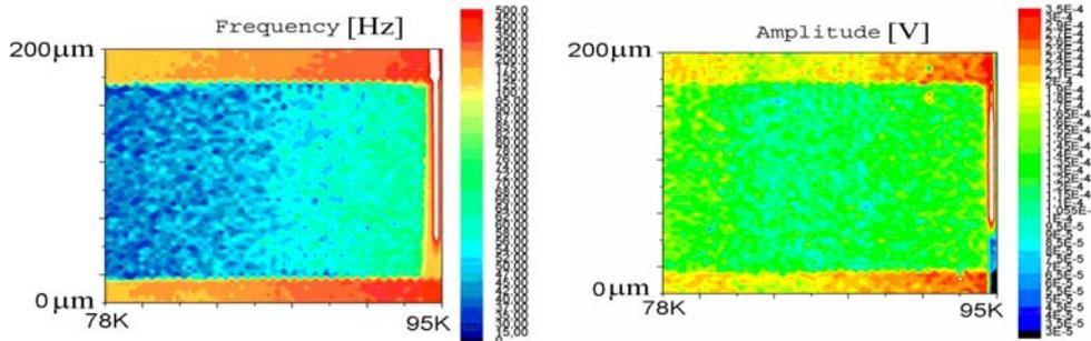
Fig. 3. Frequency shift (upper image) and amplitude change (bottom) of the SFCO-method based testing TD-oscillator, registered at the phase transition from the superconductive ( $T \sim 78\text{ K}$ ) to normal ( $T \sim 95\text{ K}$ ) of about  $160\ \mu\text{m}$  wide (vertical) HTS thin-film-bridge sample of the  $\text{YBa}_2\text{Cu}_3\text{O}_y$  composition.
