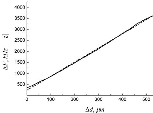
Fig. 3. Calibration curve of the thickness measuring prototype.
