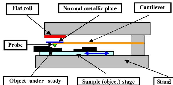
Fig. 2. Schematics of the created prototype device, based on our new idea for measuring the thicknesses of the films and tapes.
