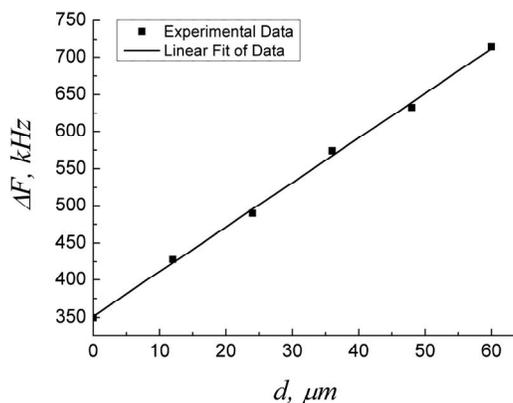
Fig. 4. Test results by use of different depth mylar tapes:  $d = 12, 24, 36, 48$  and  $60 \mu\text{m}$ .
