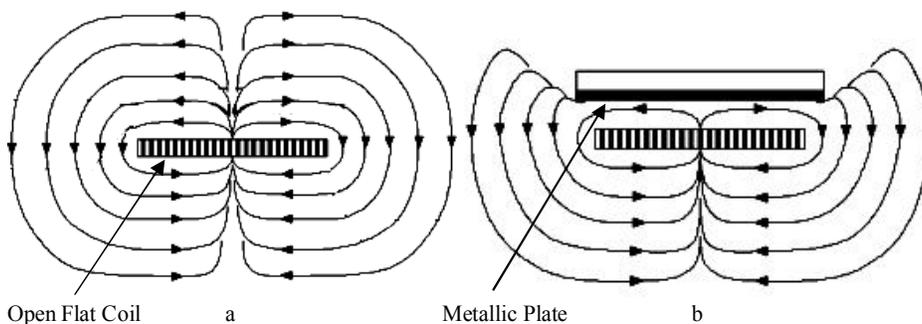
Fig. 1. Principle of operation of the single-layer flat pick-up (detecting) coil based oscillator (SFCO) technique [7–8].
