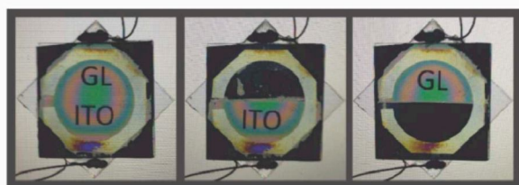
Images of the Graphene-ITO hybrid LC cell, obtained between crossed polarizers: voltage not applied (a), voltage applied to LC cell with graphene electrodes (b), voltage applied to LC cell with ITO electrodes (c).
